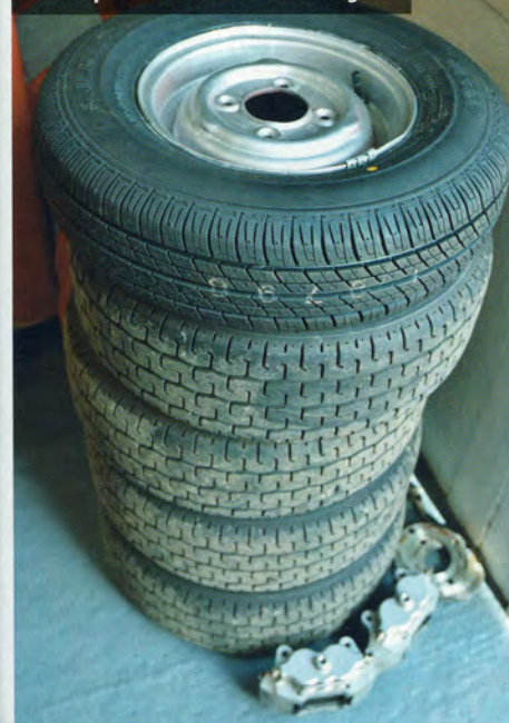
The car came with Rose Petals, four-pot callipers and a regular steel spare - these will be changed.
