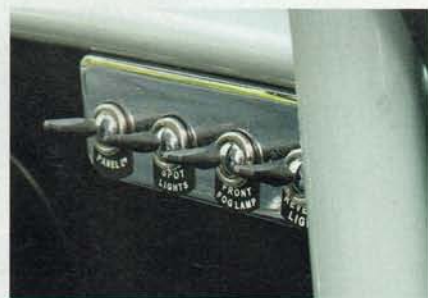
Lucas switch panel contains lettering usually found on many classic Land Rovers.
