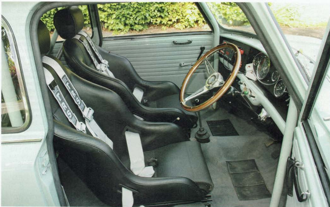
Rally-style interior includes Cobra Classic RSR high-back front buckets, FIA-approved harnesses and a Safety Devices six-point cage. Narrow Cobra Classic RSR seats provide enough room to fit runners and to actually use them. eBay Riley centre badge was the right size for the centre of the wood-rim steering wheel.
