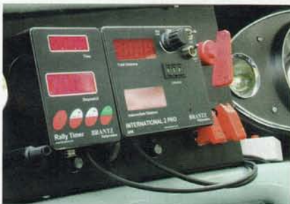
Period-looking Brantz tripmeter and stopwatch are located in front of the navigator's seat.
