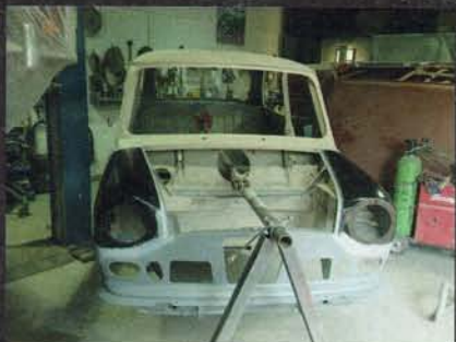
The entire front end was wisely replaced because corrosion had got the better of most of the metal.
